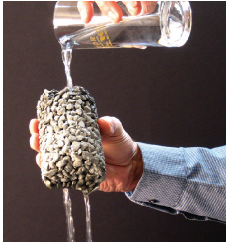
The structural backfill that meets Anchor Wall Systems, Inc.'s specifications allows water to drain behind the wall.
